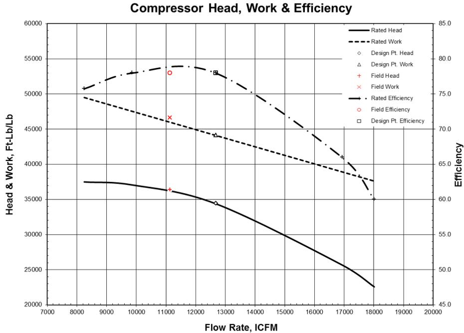
Figure 1, Natural gas compressor performance. Note that the operating data has been corrected for speed using fan laws. Also note that the work input is close to the predicted values, thus the performance values can be deemed reliable.
