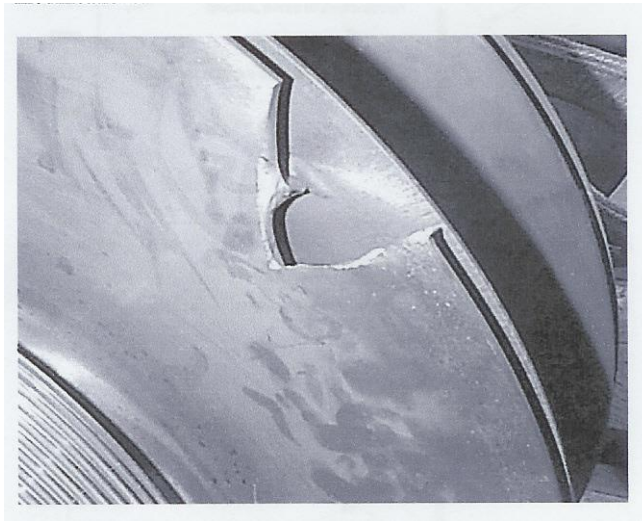
Figure #6. Impeller failure due to operation in choke with liquid ingestion.
