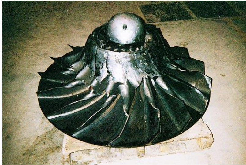
Figure #8. Impeller failure due to operation in insipient surge.
