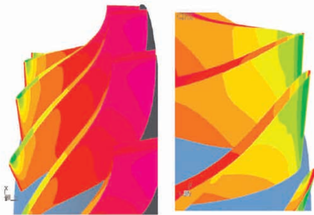
Figure 12. Static Pressure Load on High Flow Coefficient Impeller Operating at Design Flow.
