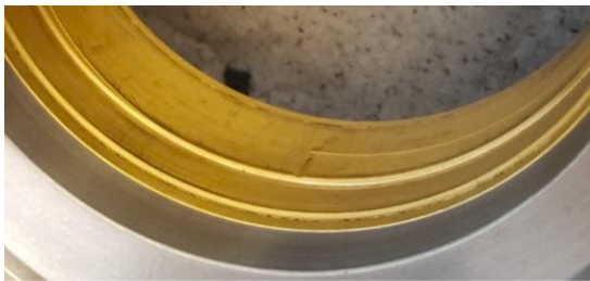
Figure 1. Photo of seal after three and one half years of rough duty. Note some scuffing marks but dimensionally per spec.
